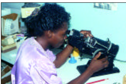
Recording the spectacle lens powers using the focimeter
